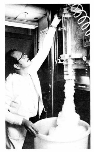
INVENTOR PETE RAND (1813) creates a batch of his new aqueous foam with laboratory apparatus. The new foam, basically soap bubbles, was developed for safeguards applications, but its stability and long life have led to agricultural and other possible applications.
